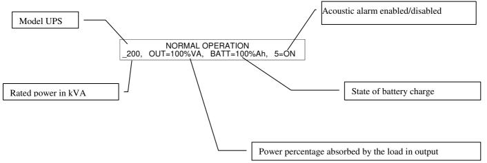
The message OUT changes to BY when the load is not powered from the inverter (normal operation) but from the mains through the by-pass line.
