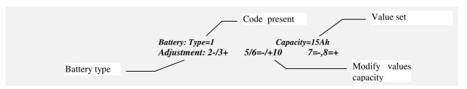
On first installation the rated capacity value of the connected battery must be inserted; this value is usually printed on the battery container.
