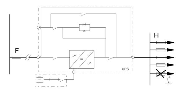
In order to select the correct protection devices to be inserted downstream of the UPS, the following two operating modes have to be taken into consideration: *mains power supply* and *battery power supply*.
