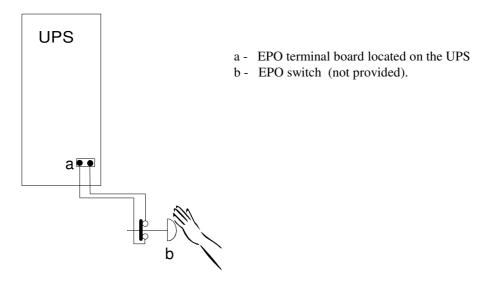
On the UPS, the jumper on the EPO terminals (page 18) must be removed, and the wires from the auxiliary contact of the button must be connected in place of the jumper.
