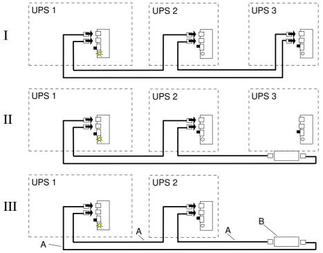
A)UPS parallel cable type RJ45
