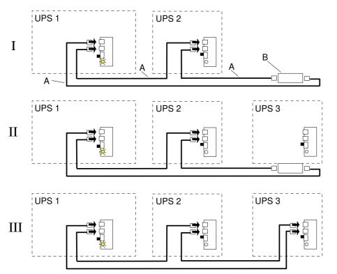
A)UPS parallel cable type RJ45
