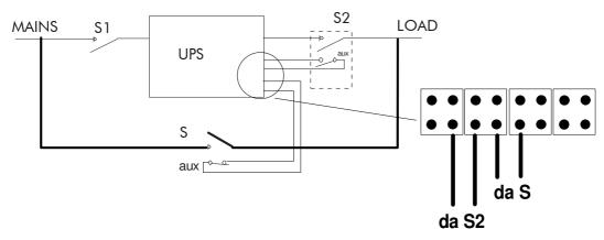
Additional output disconnector S2, additional disconnector S of the external maintenance by-pass. The auxiliary contacts S2 and S must be connected to terminals P and Q.
