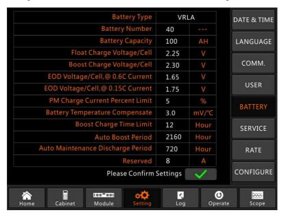
Figure 4-5 setting the period for battery auto discharge
