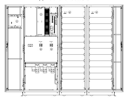
LCD control panel; SPD; Manual Bypass switch Battery cold start; Monitoring &static bypass module; Monitoring unit of 20-slot cabinet;
