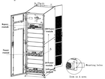
Figure 2-12 Installing power modules
