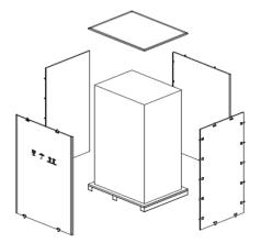
Figure 2-3 disassemble the case
