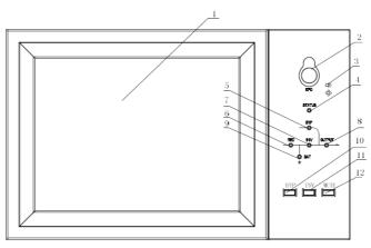
1: LCD touch screen2: EPO switch3: Audible Alarm (Buzzer)4: Status indicator5: Bypass indicator6: Rectifier indicator7: Inverter indicator8: Load indicator9: Battery indicator10: Bypass transfer11: Inverter transfer12: Mute
