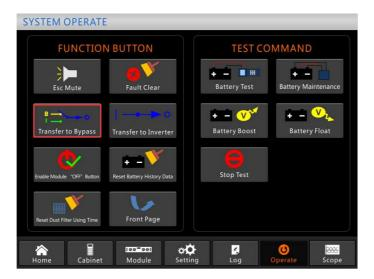
The operation interface for transferring to bypass
