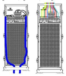
Figure 2-14 Cable entry for 6-slot cabinet
