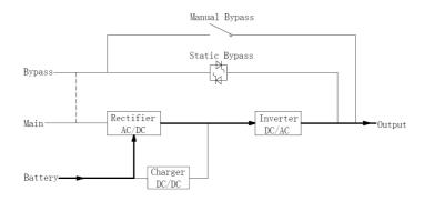
Figure 1-8 Battery Mode operation diagram
