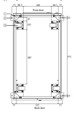
(a) 6-slot and 10-slot cabinet (Bottom view, unit: mm)
