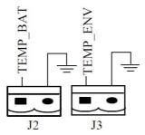
Figure 2-22 J2 and J3 for temperature detecting
