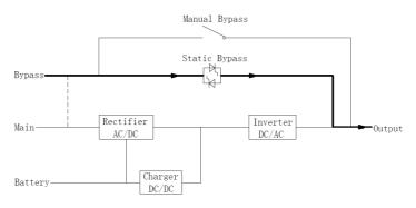
Figure 1-9 Bypass mode operation diagram
