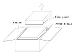
Figure 2-7 remove the foam cover
