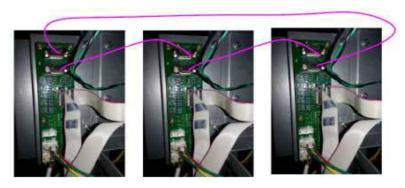
The signal cable connection for 3 UPSs in parallel
