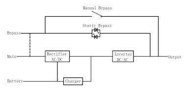
Figure 1-4 6-Slot and 10-Slot UPS Block Diagram
