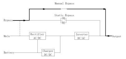
Figure 1-10 Maintenance mode operation diagram
