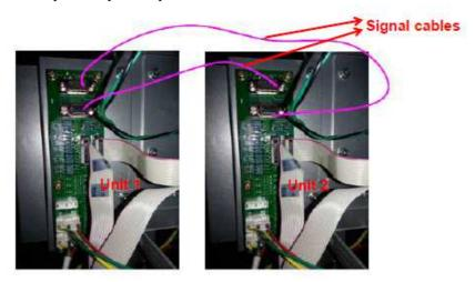
The signal cable connection for 2 UPSs in parallel
