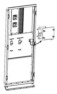
Figure 5-1 the position of inner control neutral cable
