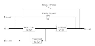
Figure 1-7 Normal mode operation diagram
