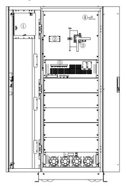
LCD control panel; SPD (optional); Manual Bypass switch Battery cold start;
