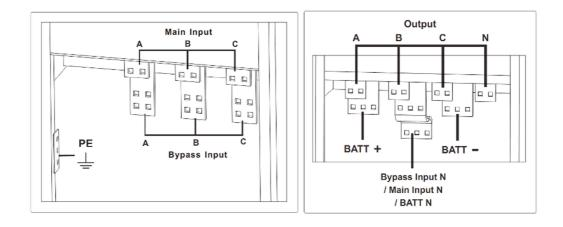
Figure 2-19 20-slot connections terminals
