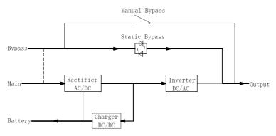
Figure 1-11 ECO Mode operation diagram
