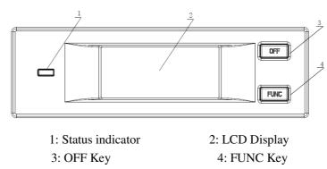
Figure 3-1 Control and display panel for power module
