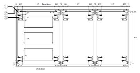
(b) 20-slot cabinet (Bottom view, unit: mm)
