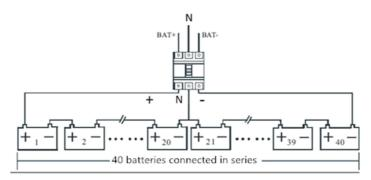
Figure 2-13 Battery string wiring diagram
