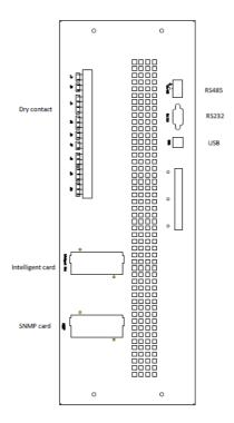
Figure 2-21 Dry contact &communication interface for 20-slot cabinet The UPS can accept the external dry contact signal and send out the dry contact signal, through the phoenix terminal ports. The cables connected to the dry contact terminals must be separated from power cables. Moreover, these cables should be double insulated with a typical 0.5 to 1.5mm² cross-section areas for a maximum connection length between 25 and 50meters.
