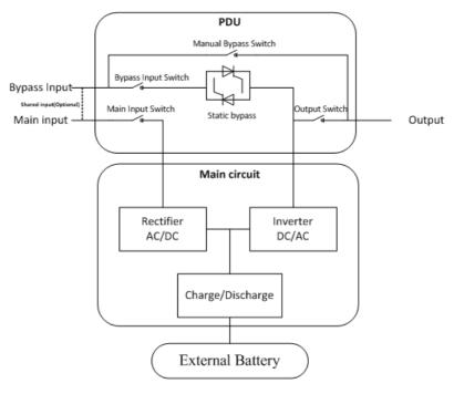
Figure 1-5 20-slot UPS Block Diagram
