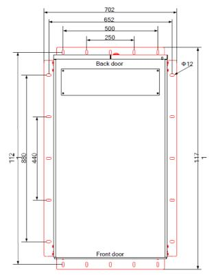
Figure 2-9 Anti-seismic Kits and mounting holes (Top view)
