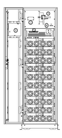
LCD control panel; SPD; Manual Bypass switch Battery cold start; Monitoring &static bypass module
