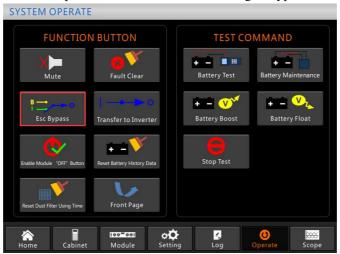
The operation interface for escaping bypass
