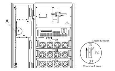
Figure 4-3 enabling the switch
