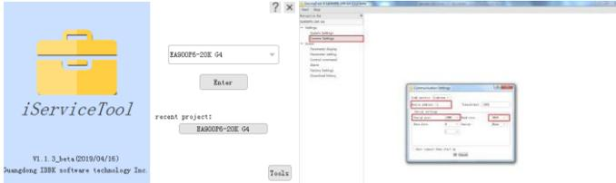
2. Enter in menu “Settings”, set “device address” as “1” and “baud rate” as “9600”, select the right serial port in menu “Communication Setting”. Click “OK” to connect UPS
