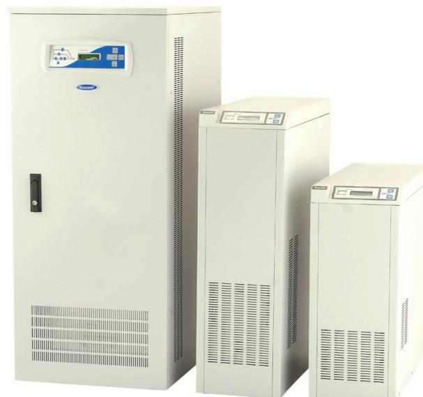
XT200 Online UPS are microprocessor controlled, full sine output uninterruptible power supplies produced with PWM (Pulse width modulation) and IGBT technologies. It provides uninterrupted energy for local networks, communication systems, sensitive medical devices, smart engineering measuring devices and industrial automation systems by guaranteeing safe operation thanks to its built-in inverter isolation transformer.
