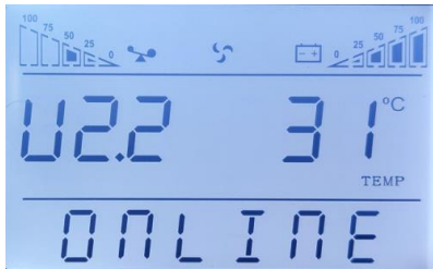
Page 4: Display UPS software version and temperature information
