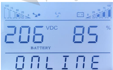
Page 6: Display UPS battery voltage, battery capacity percentage
