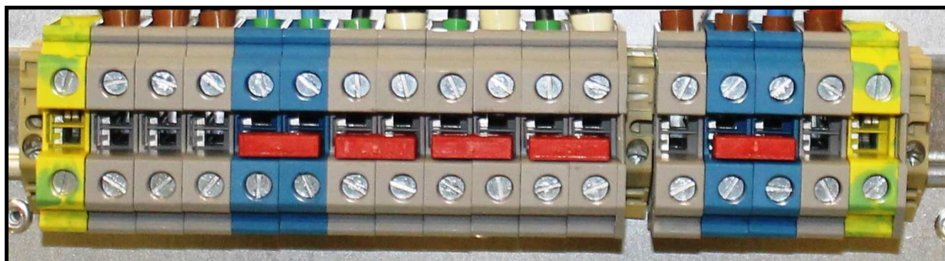
Figure 2.2 10-15-20-30 kVA Cable Connection
