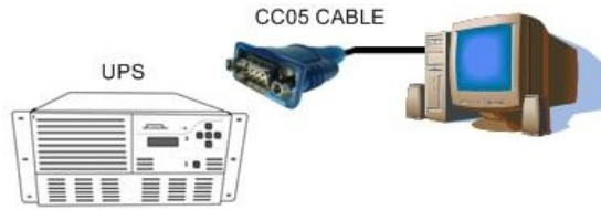
Figure 11: RS232 data connection
