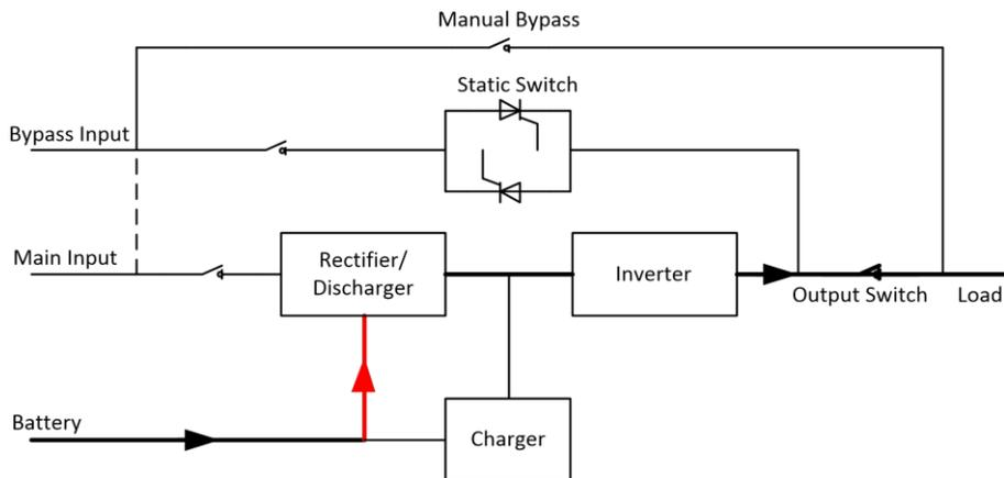
Fig 2-3 Battery mode operation diagram
