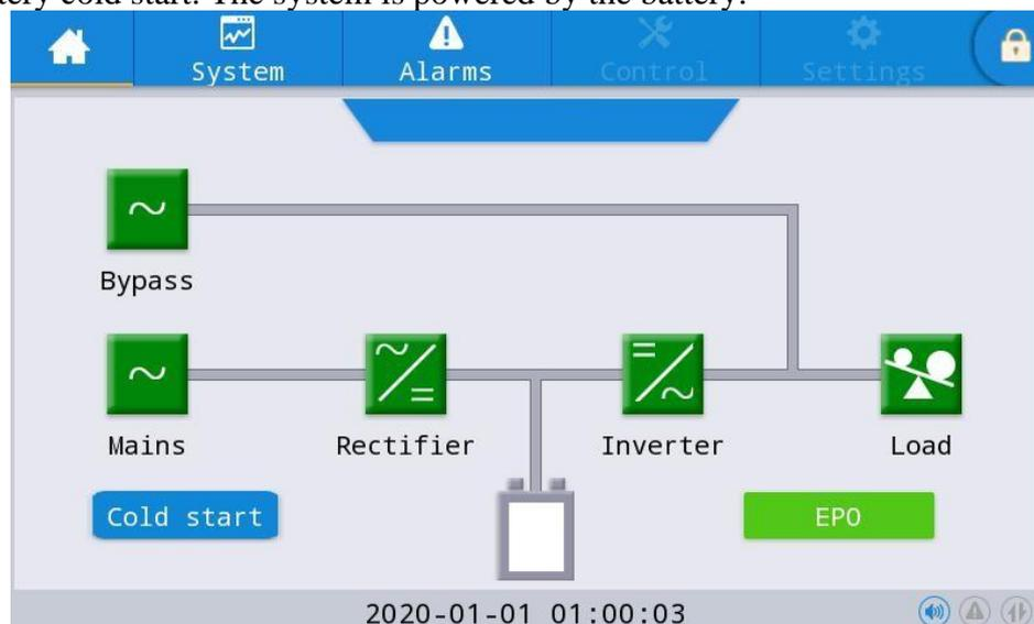
3. After that, Press the button for **cold start** on the LCD, The system is starting up following steps 3 in section 5.1.1 and the system transfers to battery mode in 30S.
