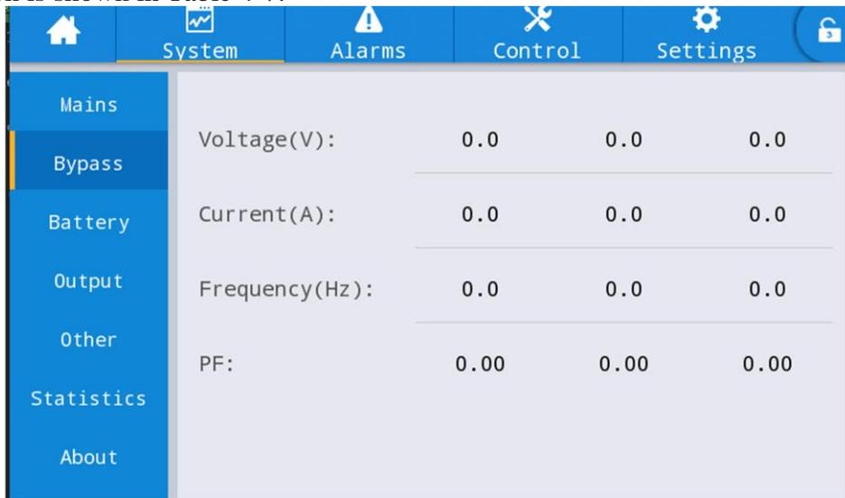
Fig. 4-5 Bypass interface
