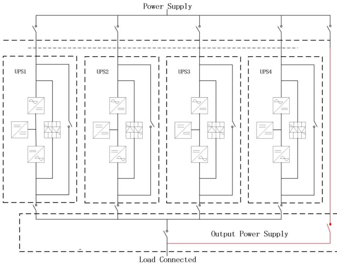
Fig. 5-4 Parallel diagram
