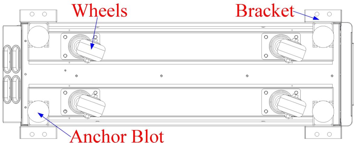
Fig.3-1 Supporting structure (Bottom view)
