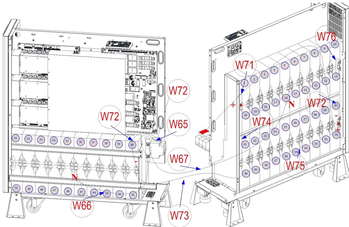
3. Connect the battery cable according to the series number
