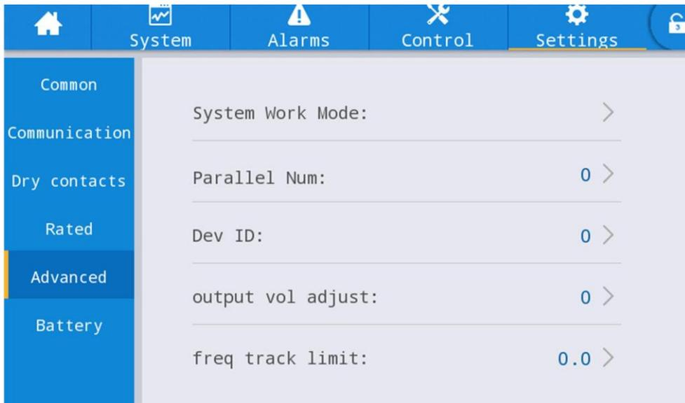
Set “**System Work Mode**” to “**Parallel mode**”, and set the “**Parallel Num**” to the number of units in parallel. For the setting of **device ID** with a system of 3 units in parallel, for example, set the number from 0 to 2 for these 3 units accordingly.
