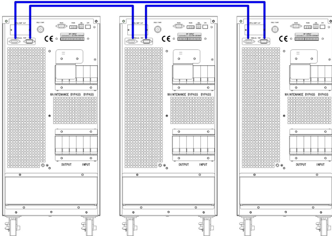
Fig.5-5 Parallel connection
