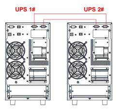
Fig 2-3: 2 UPS Paralleled System
