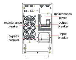
Fig 4-1: Maintenance bypass
