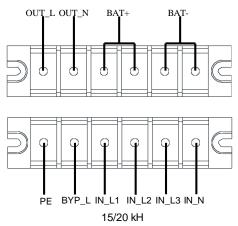
Fig 2-1: Terminal Block Wiring Diagram
