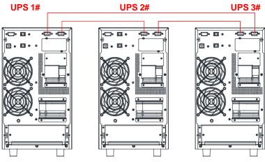
Fig 2-4: 3 UPS Paralleled System'
