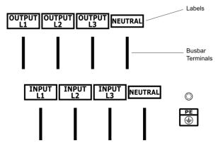
• Compression cable lugs must be used for connecting the conductors to busbar terminals.
