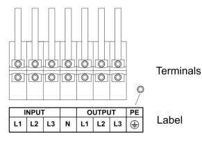
Above image showing terminals of a standard device. In standard devices there is only one neutral terminal. Connect input and output neutral conductors together to this common neutral terminal.
