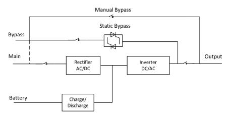
Figure 2-1 UPS Conceptual Diagram
