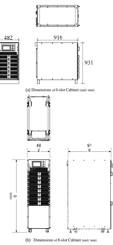
Figure 3-1 Dimensions of Cabinet (unit: mm)
