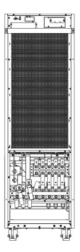
(b) 8 slot UPS Cabinet structure (back view)
