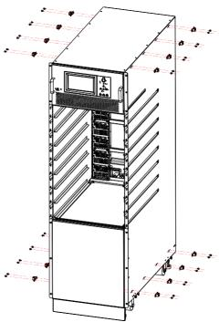
Figure 3-8 Remove bracket for cabinet side door
