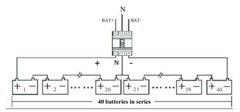
Figure 3-13 Battery string wiring diagram
