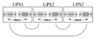
Figure 5-7 Parallel connection
