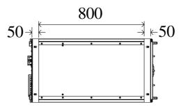
(a) Supporting structure of 6-slot Cabinet (Bottom view, unit: mm)
