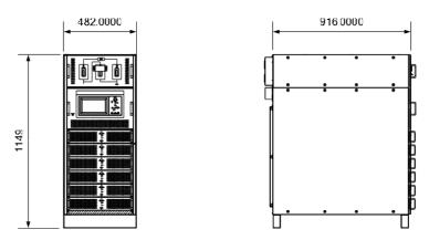
Figure 0-1 Size diagram of 6 module cabinet with PDU
