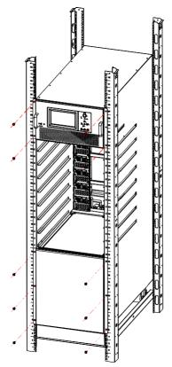
Figure 3-10 Load the UPS into the server cabinet
