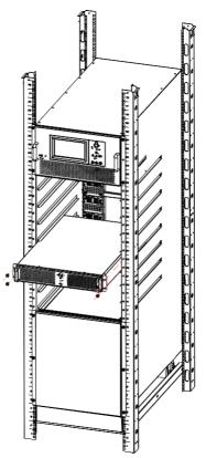
Figure 3-11 Insert module to cabinet
