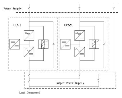
Figure 5-6 Parallel diagram
