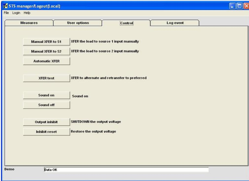
**CONTROL menu:** the user can perform manual or automatic switching from the preferred source to the alternative source and vice versa as well as send other auxiliary commands.
