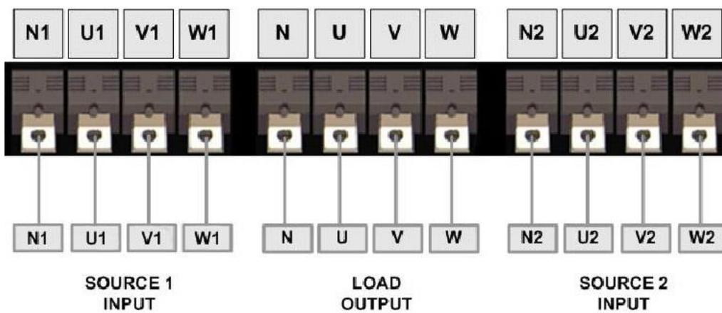
OUTPUT NEUTRAL IS CONNECTED TO CURRENT SOURCE NEUTRAL
