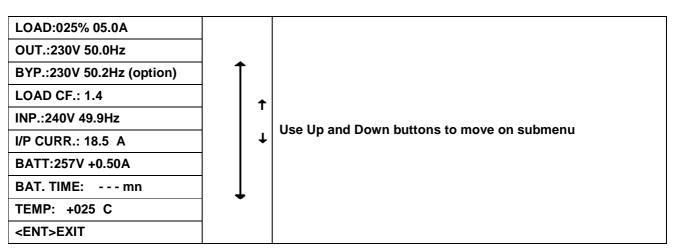
From this menu users can see all measured parameters of the UPS. The submenu items are listed as follows by order of appearance.
