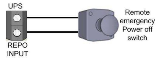
This isolated input is used to turn off the UPS remotely in case of emergency. The UPS is supplied from the factory with REPO terminals open-circuited (see "View of the UPS connections") if those two (NO) terminals are shorted, UPS shuts-down the output voltage.
