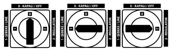
Fig.-7 Regulator Pako Switch Working Positions
