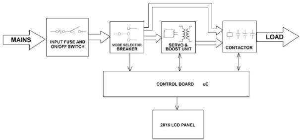
Fig.-3 Regulator block diagram
