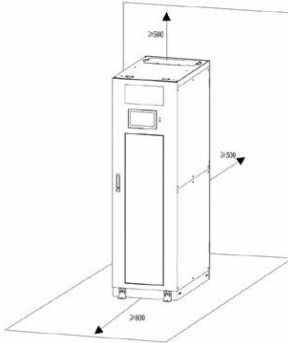
Figure 3-2 Space reserved for the cabinet (Unit: mm)
