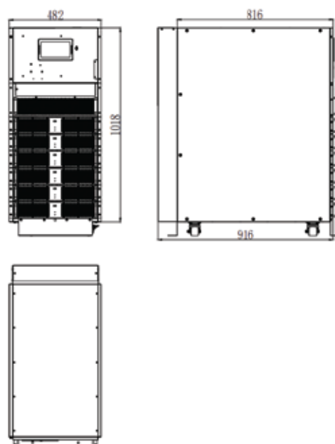
(a) The size diagram of the 4-slot cabinet (Unit:mm)
