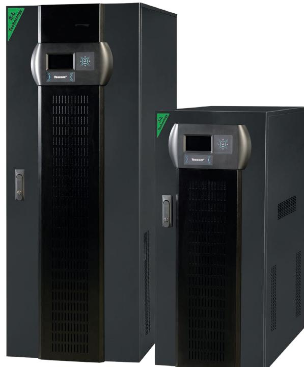
TESCOM DS300C Frequency Converters are produced to provide the energy for your devices, which are powered by AC voltage and requires different frequency ranges. Our converters, which have many usage areas, mainly in maritime, aviation, industrial equipments and military applications, are designed for continuous operation with PWM and IGBT technology and convert 50Hz or 60Hz mains energy to 50Hz, 60Hz or 400Hz energy to supply your critical loads.
