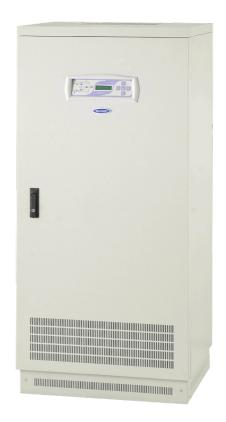
STS 3000 3 phase, 3 pole static transfer switch transfers uninterruptedly critical loads to either of two independent AC power lines. The system monitors two AC inputs. If any of them goes out of the specified tolerance, it transfers the critical load to the other. By increasing the energy quality of the systems used with STS 3000, while reducing the effects of interference and short interruptions, a backup power system is gained.
