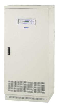
STS 4000 3 phase, 4 pole static transfer switch transfers uninterruptedly critical loads to either of two independent AC power lines. The system monitors two AC inputs. If any of them goes out of the specified tolerance, it transfers the critical load to the other. By increasing the energy quality of the systems used with STS 4000, while reducing the effects of interference and short interruptions, a backup power system is gained.
